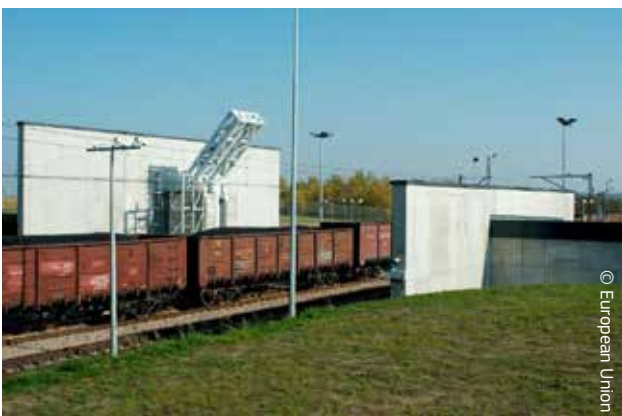
Scanner used to check trains at the border between Poland and Ukraine.
